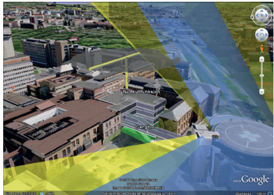
DP05 model in Google Earth with helicopter flight corridor. Source HENT using Onuma and SketchUp.
